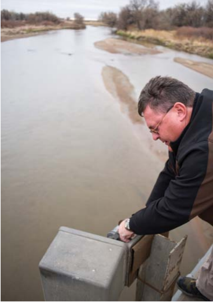
ROAD WARRIOR: Brent Schantz (BA-93) uses a wire weight to get a stage level at the Kersey gauging station. It takes 2 ½ hours to drive across his districts, which include the South Platte River and the gauge house (opposite page) overlooking Bijou Ditch, east of Kersey.
