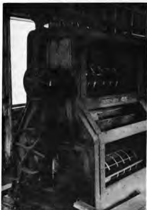
Photo courtesy of Betty Curry Angle view showing the sifting reels which held the “silks.”
