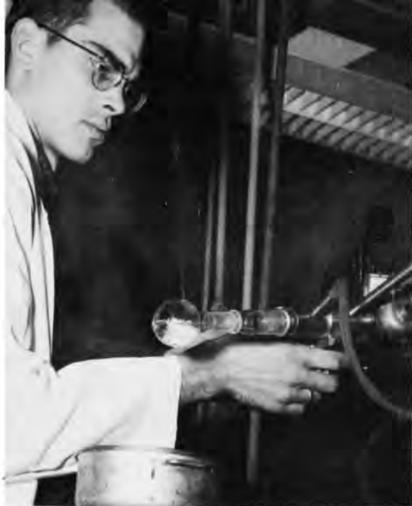
A student uses a flash evaporator in an organic chemistry laboratory.
