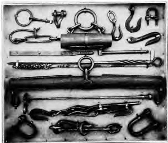
Work in Iron Done by Students in Forging
