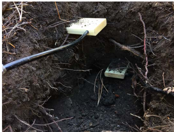
Figure 6. Soil moisture sensors installed at 5 cm and 20 cm depth.
