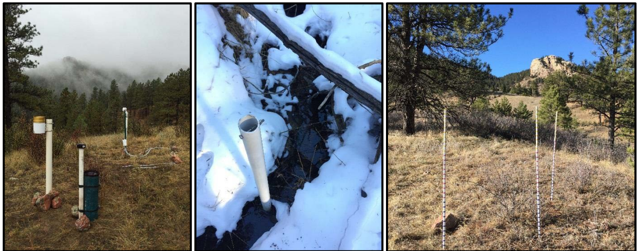
Figure 2. Precipitation and soil moisture instrumentation at Mill Creek (left), water level instrumentation at Lazy D (center), and snow poles for time lapse camera measurements of snow depth at Mill Creek (right).
