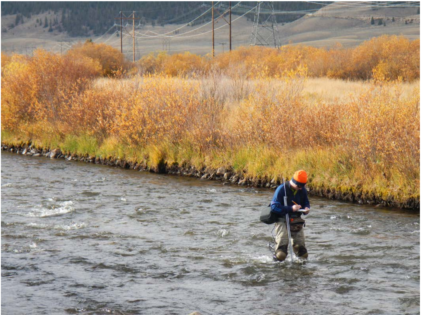
Stream flow measurements at the upper Arkansas River. Photo credit: Sam Duggan
