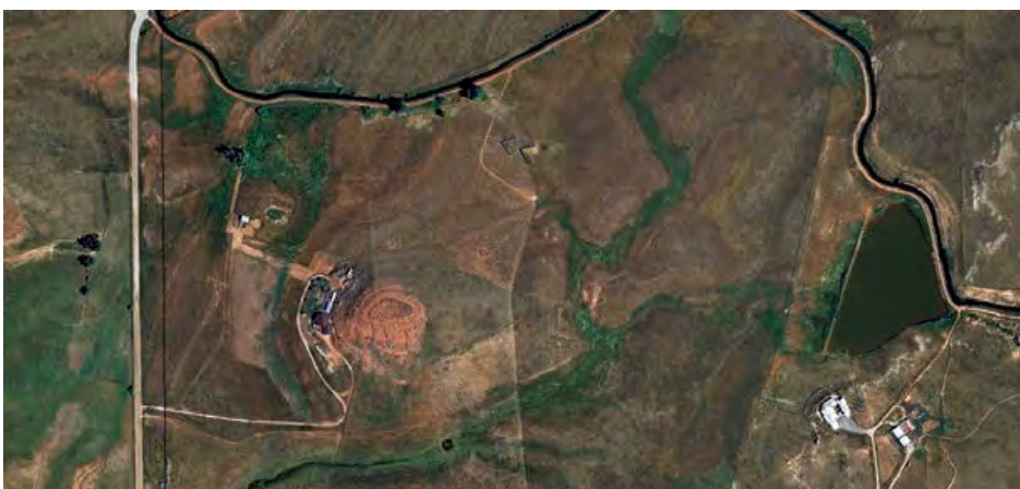
Aerial image of an irrigation canal transporting water across a semi-arid landscape. Various points of water leakage in the canal lead to the flow of water down the landscape, converging to create wetland habitat in topographic depressions.
