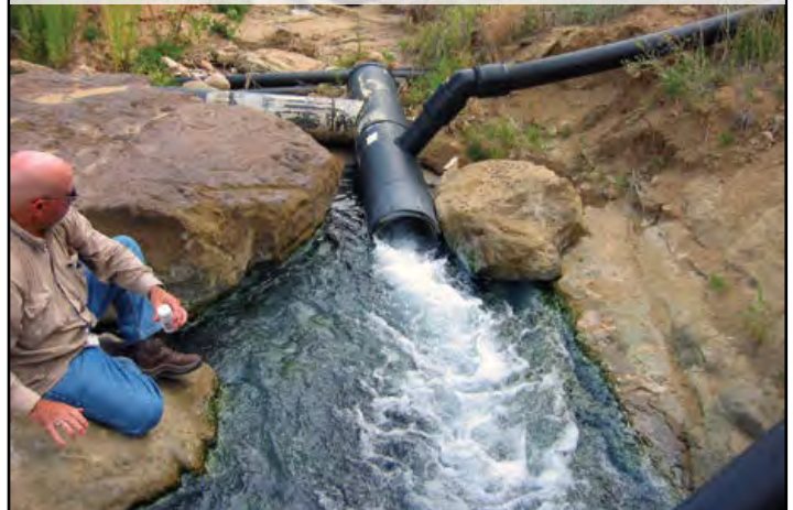
Sampling CBM discharge water in the Raton Basin of Colorado. Photo by Troy Bauder, Colorado State University
