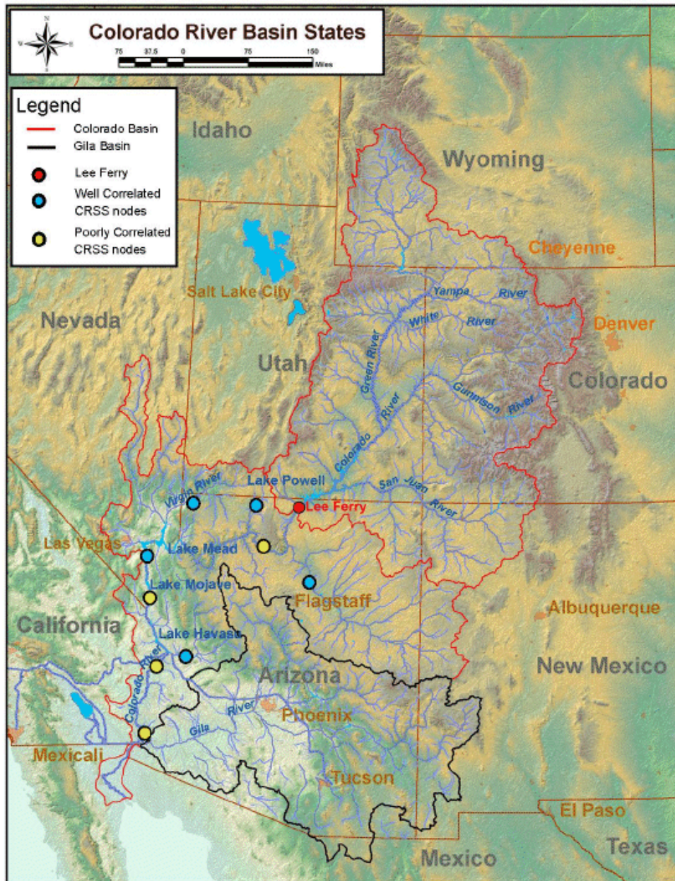
Figure 1. Colorado River Basin (CRB). The basin is divided at Lee Ferry (red dot) for legal and management purposes into an Upper Basin and Lower Basin (red boundaries). The watershed of the Gila River is outlined in black. USBR’s 9 CRSS model nodes in the Lower Basin are shown as blue and yellow dots. The intervening flows at the 5 blue nodes are well-correlated with precipitation while the 4 yellow nodes are not. We used only the 5 blue nodes in our Lower Colorado mainstem flow reconstruction.
