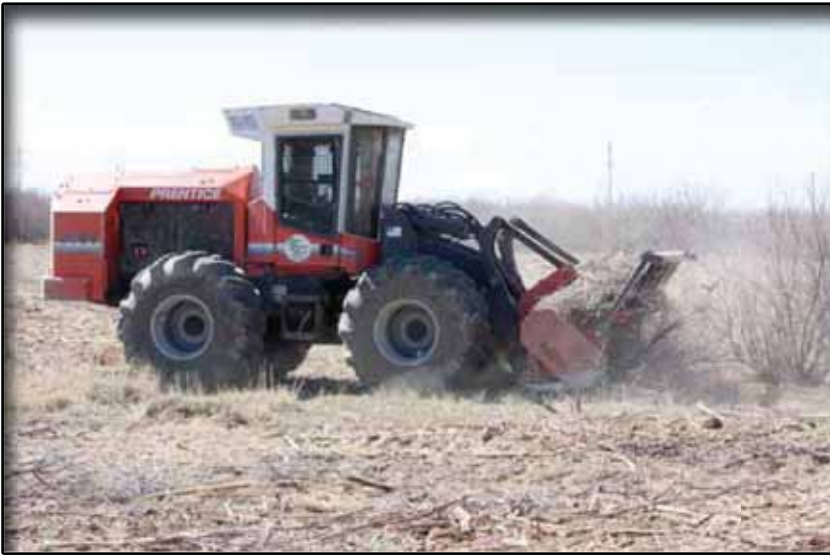
Figure 2. Prentice Hydro-Ax equipped with a Fecon mulching head being used to shred the aboveground portion of tamarisk trees.
