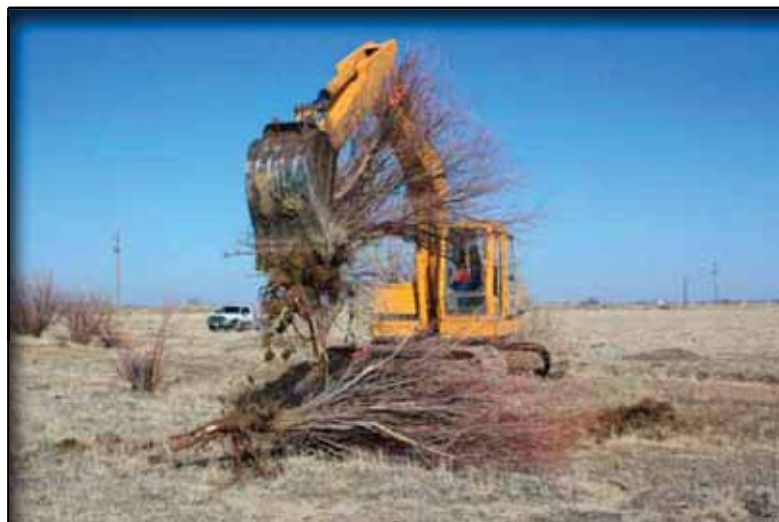
Figure 1. Track hoe equipped with thumbed bucket being used to excavate entire, living tamarisk trees
