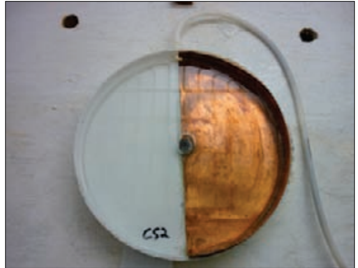
This image shows a 21.5-cm diameter PVC arena that was used to evaluate the New Zealand mudsnails' response to various copper-based materials. (Courtesy of Scott Hoyer)
