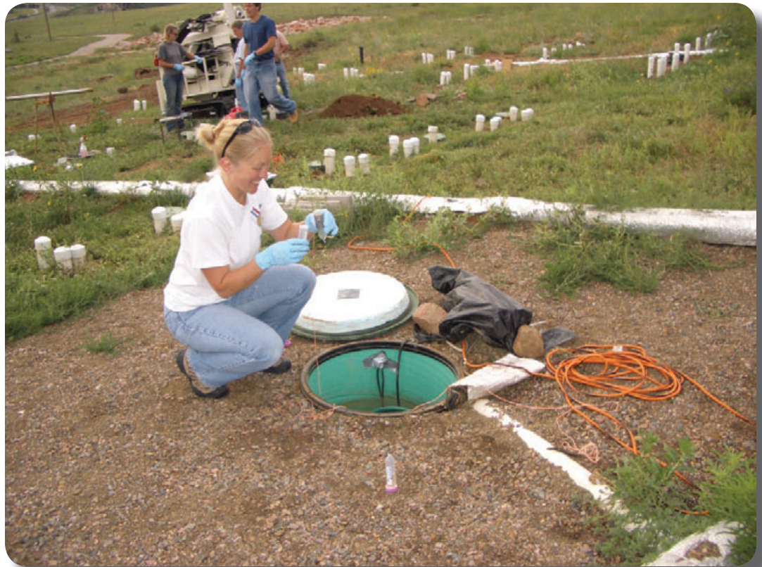
Conn sampling septic tank effluent at the Mines Park test site during a multi-component tracer test
