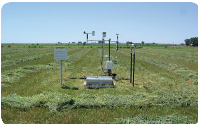
Fig 5: View of the lysimeter & meteorological instrumentation in late June '07. Photo taken by Michael Bartolo.
