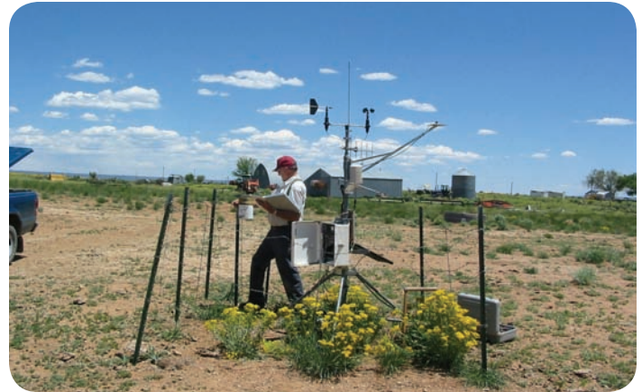
Figure 5. CoAgMet volunteer Dr. Harold Duke services Dove Creek. Due to the lack of underlying vegetations, sites like this may not be ideal for ET applications
