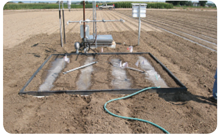
Fig 6: Water being applied to the soil monolith. Photo taken by Michael Bartolo.
