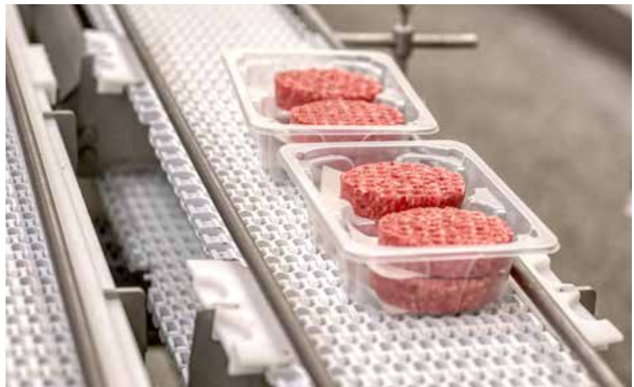
Machine-formed beef patties move on a packaging conveyor in a meat processing facility. Photo © nordroden/adobe.stock.com.
