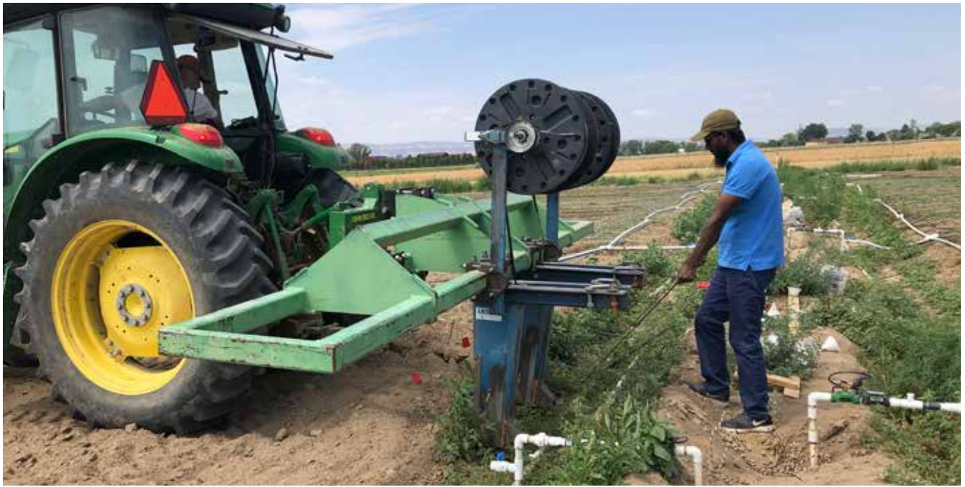
Azmal Hossan assists his mentor, Dr. Perry Cabot, place irrigation drip tape underground at CSU's Western Colorado Research Center-Grand Valley. Photo by Cordelia Anderson.
