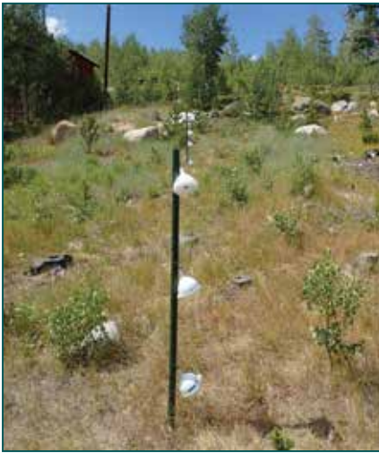
Figure 3: T-posts with double-funnel radiation shields holding the temperature sensors along the hillslope, at the CSU-MC. Photo by Dr. Steven Fassnacht.
