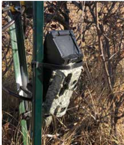
Figure 3. A game camera was installed next to and aimed toward an ephemeral channel in West Stroh Gulch. A staff gauge installed in the center of the channel provides an approximation of flow depth. Photo by Stacy Wilson.
