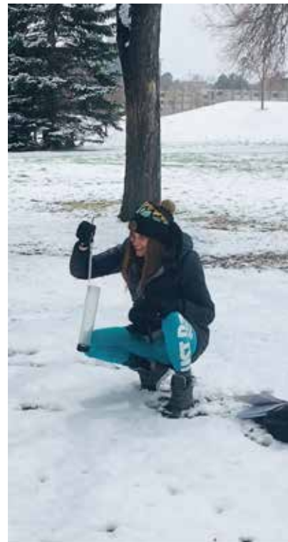
Figure 1. During an April 2020 snowfall event in Fort Collins, Marcee Meinhardt measures SWE by weighing the snow in the fresh snow sampler.
