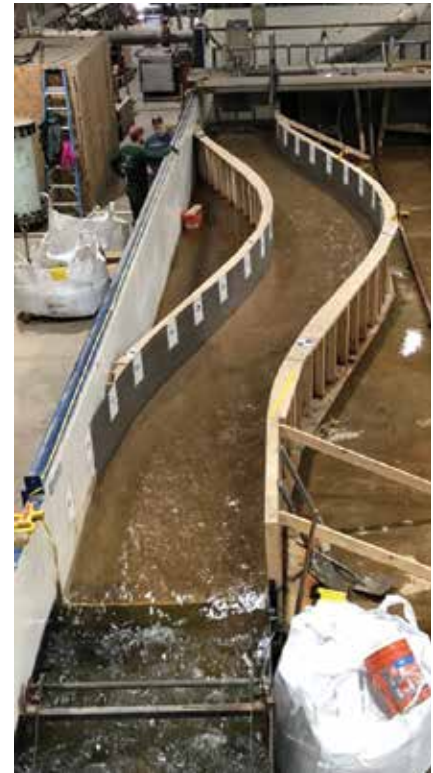
Figure 1. The single meander bend gravel-bed flume in operation at the CSU Hydraulic Laboratory.
