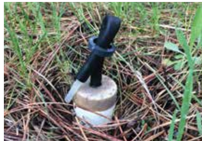
Figure 3. Tension lysimeters installed at the Mill Creek research site collect soil water following snow melt events. Photo by Alyssa Anenberg.
