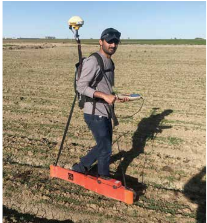
Figure 1. Image of the EM38-MK2 electromagnetic induction device, coupled with handheld computer and GPS for mapping soil salinity in a newly planted alfalfa field near Swink, Colorado.
