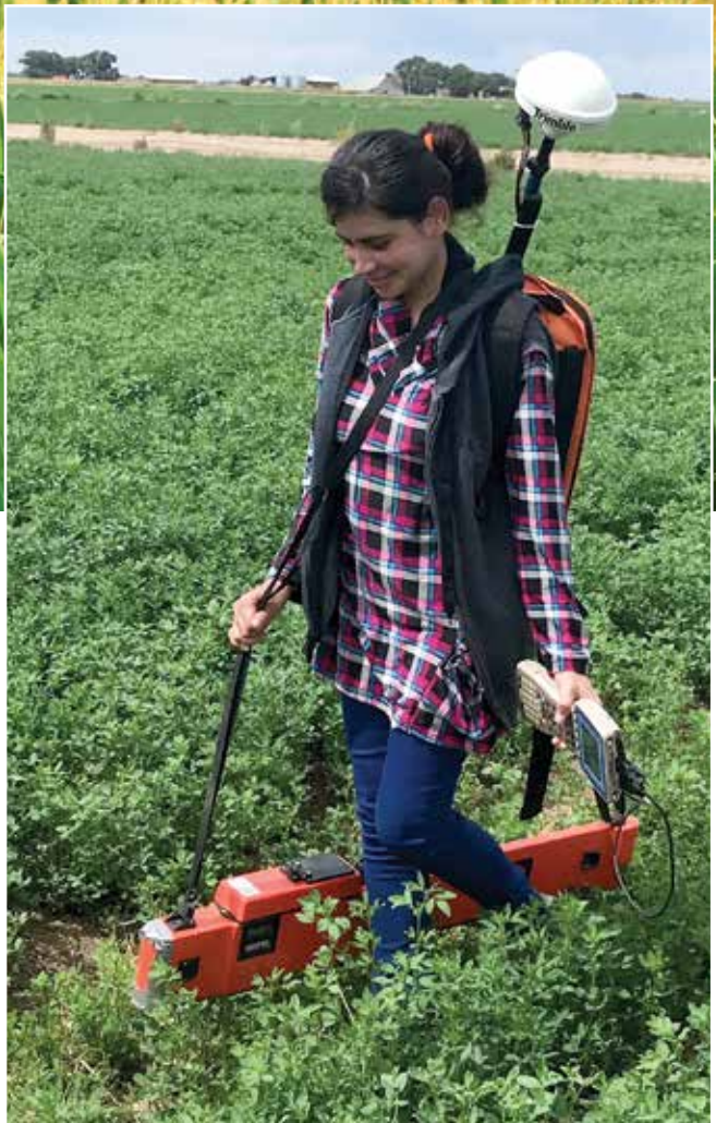
Figure 2. Kainat Kalhoro, exchange student from the US-Pakistan Center for Advanced Studies in Water, conducting an EMI survey of an alfalfa field using a Geonics EM38-MK2 meter and GPS unit. Photo by A.J. Brown.
