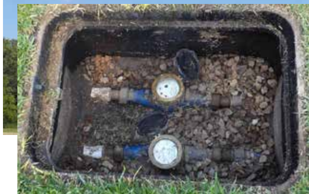
Figure 4. Water applications will be quantified for each plot using Rainbird water-flow meters (Model FM100B). Photo by Don (Wes) Dyer.
