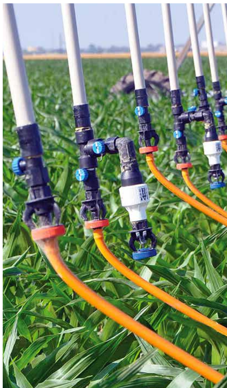
Mobile drip irrigation. Photo by Kansas State Research and Extension.
