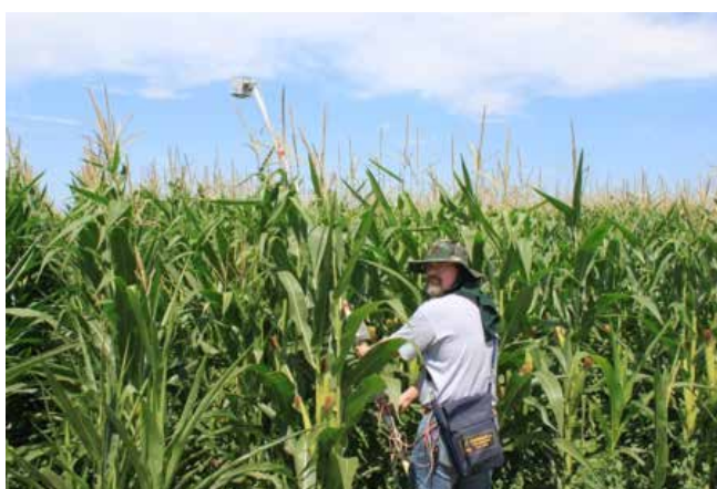
Figure 4. Handheld multispectral radiometer taking readings over fully irrigated corn (top) and deficit irrigated corn (bottom), on 20 August 2017. Photos courtesy of Dr. José L. Chávez.
