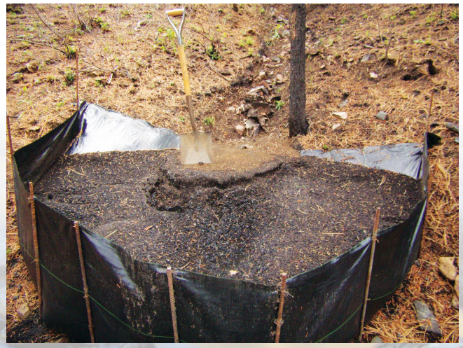
Figure 2. Sediment fence used to measure erosion after the High Park Fire. After rainstorms, researchers dug out and measured the accumulated mass. These are placed in small convergent hillslopes as indicated by the small rill leading into the sediment fence, indicating significant post-fire overland flow. Photo by Sarah Schmeer.
