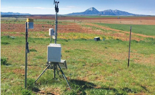
Figure 1. A typical CoAgMET weather station with a wind vane at 2 m. This photo comes from the Yellow Jacket Site in southwest Colorado. Photo by Zach Schwalbe.
