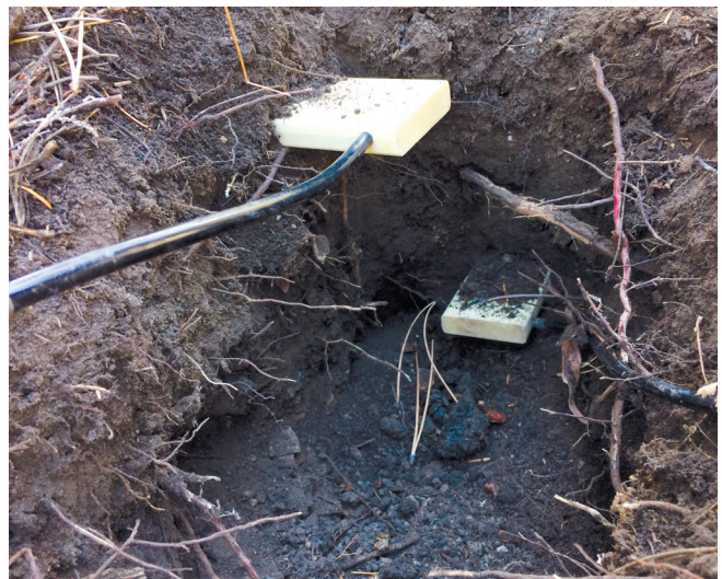
Soil moisture sensors installed at 5 and 20 cm depth.
