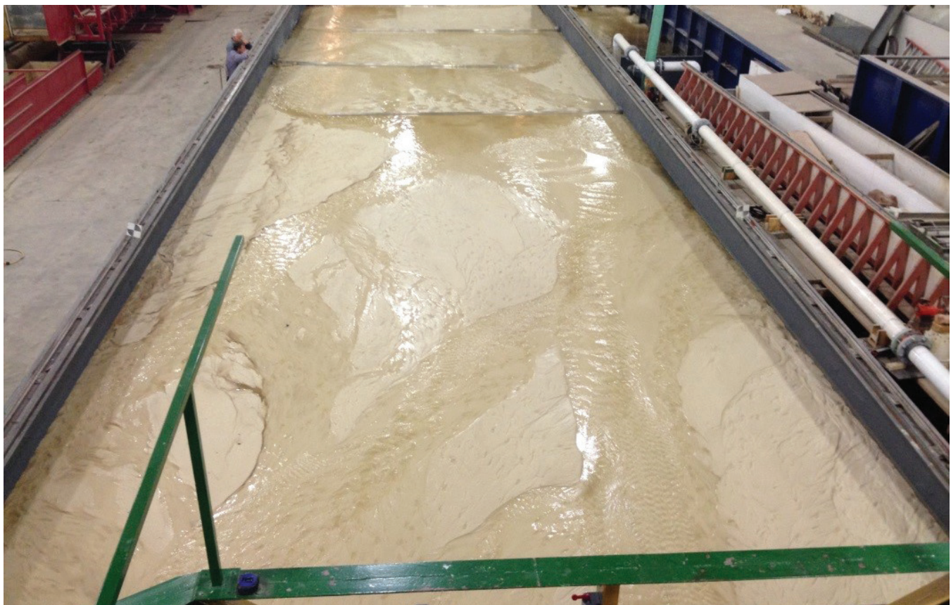
Figure 2. The 8 m by 33 m flume used to model a system of sediment-trapping structures placed in a braided-channel reach of a river that adjoins Mount Saint Helens, Washington.
