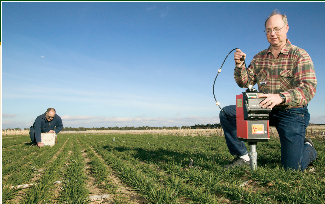
Agronomist David Nielsen (right) uses a neutron probe as technician Martin Walker uses time domain reflectometry to assess soil water used by winter wheat in an alternative crop rotation study. Courtesy Stephen R. Ausmus USDA-ARS
