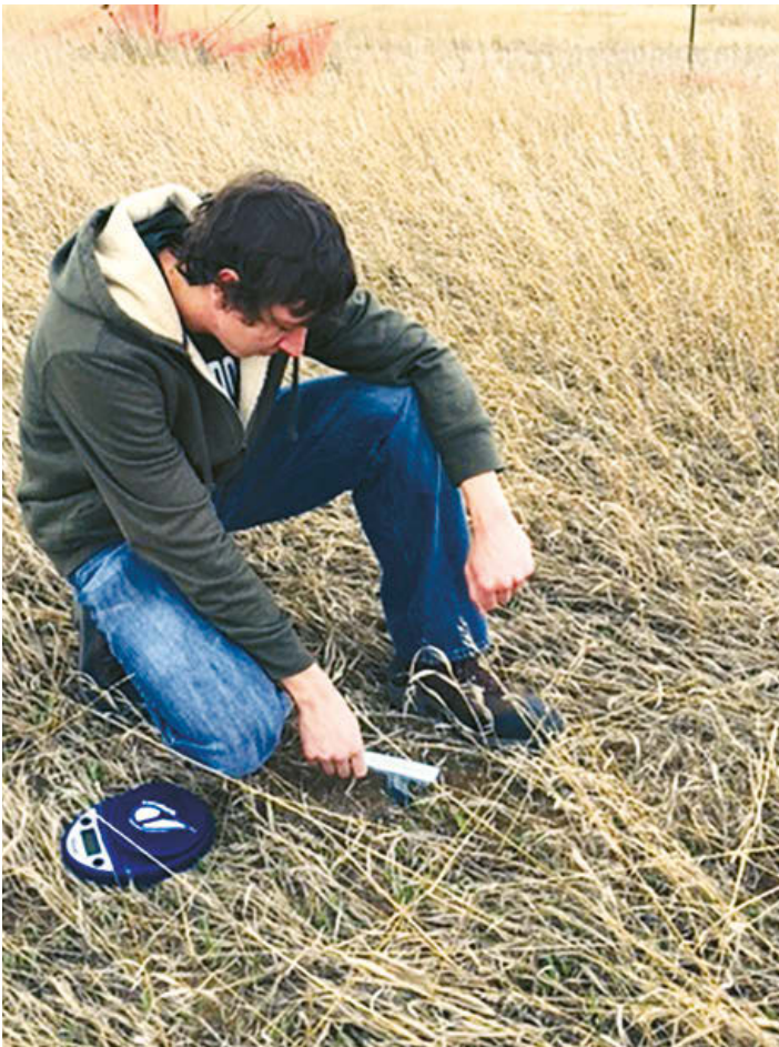
Figure 1. Peter Goble took soil cores from the Christman Field Weather Station near the CSU Department of Atmospheric Science. These soil cores were taken at various depths within the root zone, weighed, dried under a heat lamp, and weighed again to determine what percent of soil volume is water. The findings presented here were from computer models in which the root zone soil moisture field is mathematically derived. This is because soil core data are not available at high spatial or temporal extent. Ultimately, field observations like this must be used to ensure that data derived by land-atmosphere models, such as the ones used in this study, are accurate. Eastern Colorado (below), where the majority of the region's agriculture is located, was indicated by these data to be more resilient against the root zone soil moisture-temperature feedback than other areas.
