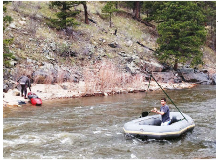
Tim Stephens and a fellow student on the Cache la Poudre River northwest of Fort Collins test a method for surveying whitewater parks that are too difficult to wade.
