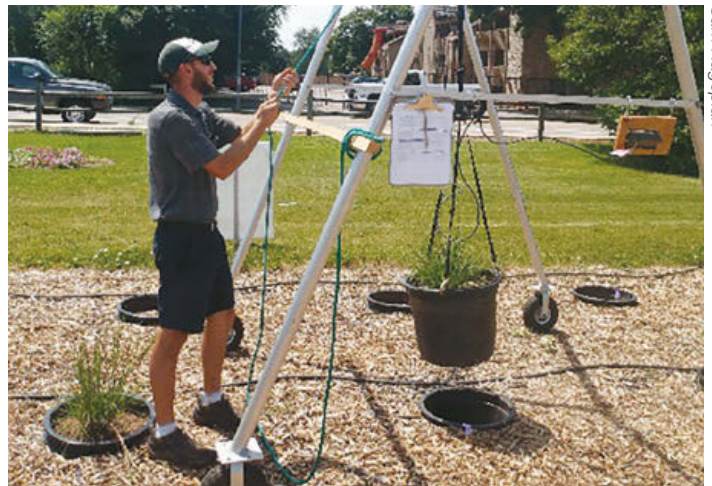
Figure 2. Sam Hagopian uses the mini-lysimeter to measure pot and plant weight during dry down periods, in which plants were dried to critical stress levels.
