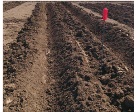
Above Left: Ph.D. student Rosemary Records (left) and Steven Fassnacht, Professor of Snow Hydrology, construct the meteorological tower. Above Right: Furrows were dug on the upwind fetch of the experimental site to induce roughness.
