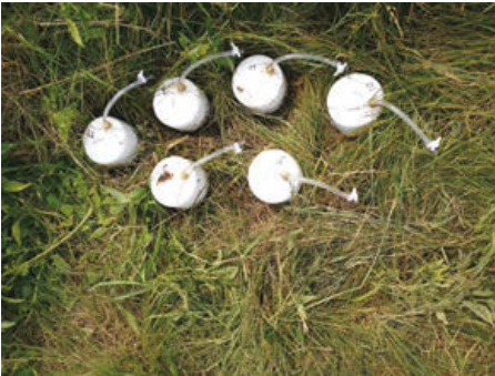
Figure 3. Soil incubation chamber in the field near Gilcrest. Notice the gas exchange port and stockcock for taking samples.
