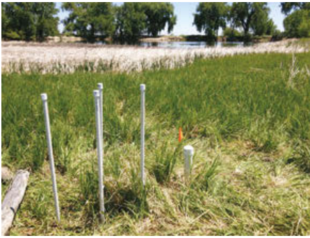
Figure 2. A groundwater well and piezometer set in a wetland near Ault, Colorado.
