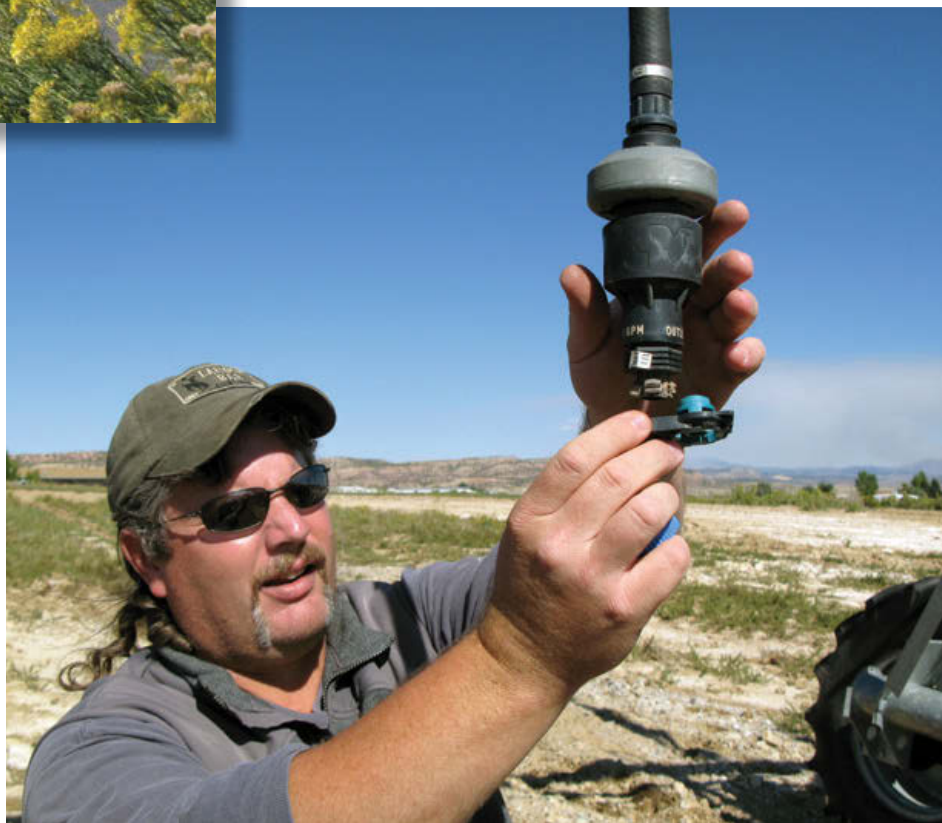
Bad experiences with the first pivot sprinklers in the 1980s have delayed adoption of newer technologies among row-crop farmers in the salt affected areas of the Upper Colorado. This producer adjusts an emitter on a more modern pivot, which runs on lower pressures—around 30 psi—producing smaller droplet sizes, which greatly improves infiltration and crop water uptake.
