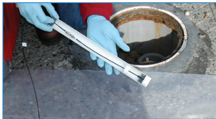
Figure 3. This device was developed to enable the biosensors to be used in groundwater monitoring wells. The plastic housing protects the sensor tip and weights in the bottom, allowing the assembly to be lowered. This apparatus has been used to measure contaminant concentrations at different depths, revealing unexpected stratifications of contamination in an aquifer.
