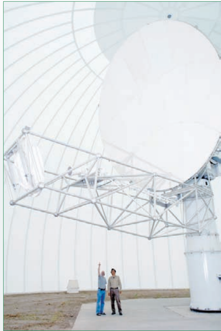
Figure 1b. The dual offset feed antenna inside the radome.
