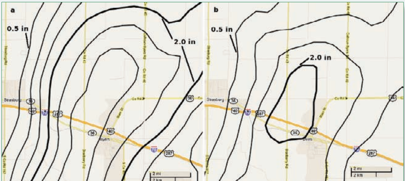
Figure 4. Rainfall accumulations in inches (outer contour is 0.5; interval is 0.5; 2.0 inch contour is darkened) calculated from CSU-CHILL data collected during the 6:15 – 8:30 p.m. MDT period on July 6, 2010. Accumulations in panel a were computed using current NWS methods that only consider reflectivity ( Z_h ). Panel b results are based on CSU procedures that combine Z_h data with the additional polarimetric information contained in the Z_{dr} and K_{dp} data.
