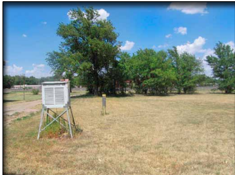
Standard NWS Cooperative station on the Eastern Plains of Colorado showing Cotton Region Shelter and 8 inch Standard Rain Gage.
