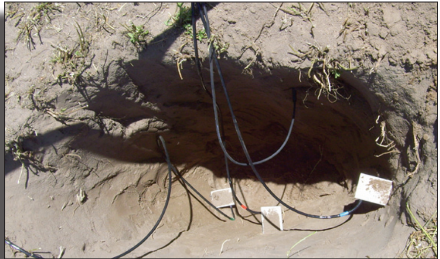
Figure 1. Soil water content reflectometer probes were installed at a depth of one, two and three feet in a sandy soil near La Salle, Colo. to monitor irrigation water management practices.
