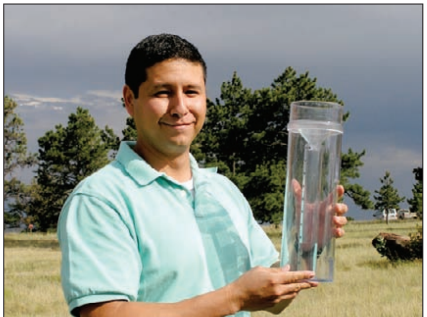
James Cano displays a rain gauge, used to measure precipitation. Accurate measures will help develop consistent data for the use of water conservation experts. Courtesy of Nolan Doesken.
