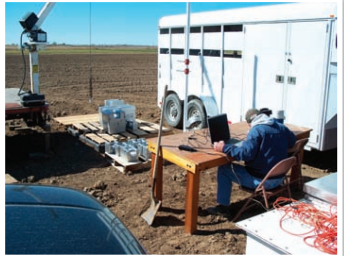
Figure 3. This image shows calibration of the reference lysimeter weighing scale. Certified weights of varying size were placed on top of the monolith to derive the relationship between load cell output and monolith tank weight. (Image courtesy of Lane Simmons)
