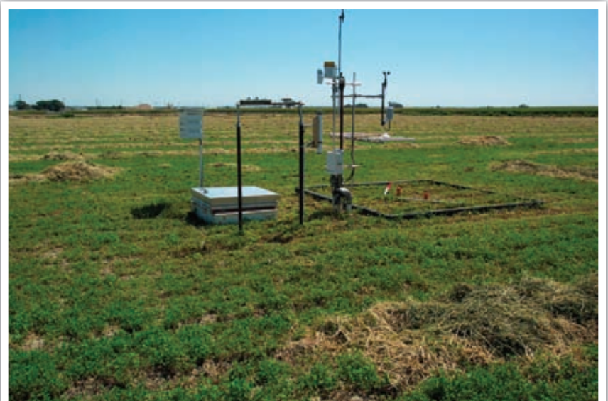
Figure 4. This view of the crop lysimeter is looking to the east. The manhole for accessing the data logger, weighing mechanism, and drainage tanks is on the left; and micrometeorological (weather) sensors are mounted above the lysimeter.
