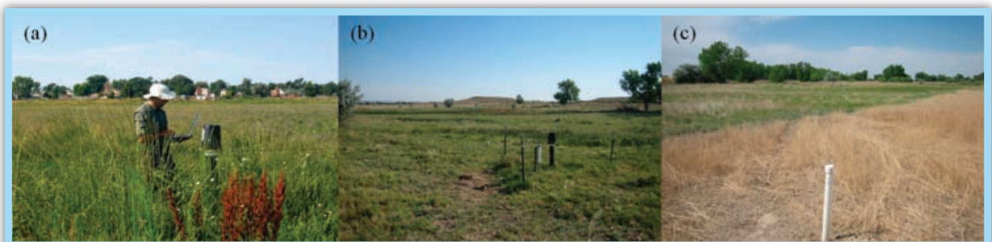
Figure 1. (a) Researcher downloading data from a rain gauge at the Swink field site, (b) Rain gauge and atmometer at the Manzanola field site, and (c) monitoring well at the Rocky Ford field site.
