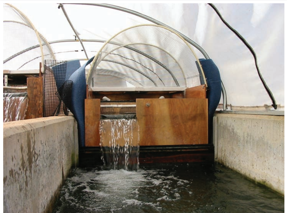
Figure 1. The Kondratieff-type artificial waterfall is used to measure the effects of waterfall height and plunge pool depth on the jumping ability of brook trout.
