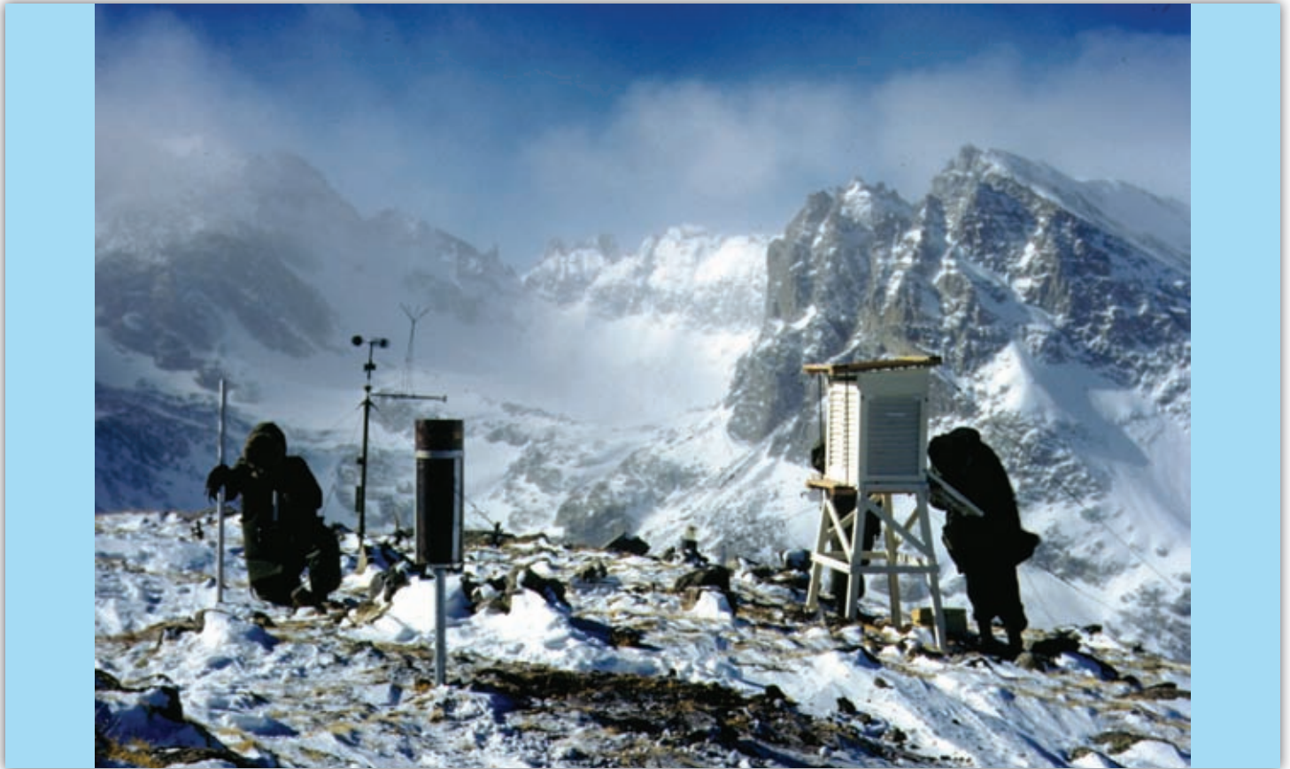
Figure 1. Maintenance work is done on a high-elevation meteorological station at the NWT LTER site in the mid-1950s (NWT LTER archive).
