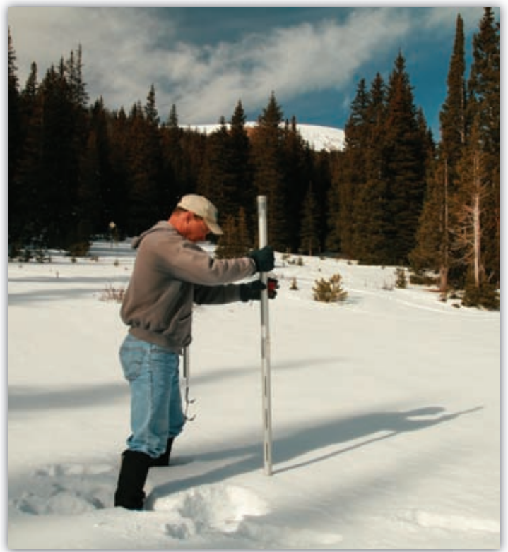
Figure 3. Todd Boldt of the USDA Natural Resources Conservation Service (NRCS) takes snow measurements at the Cameron Pass snowcourse.
