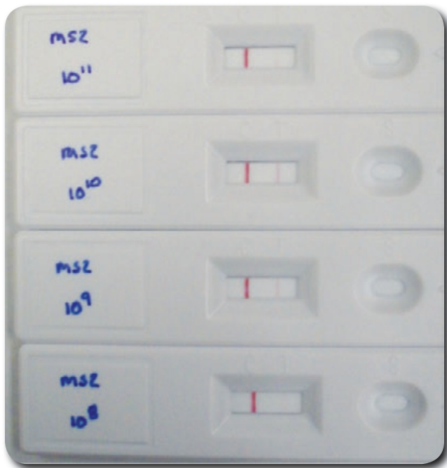
Figure 4. Lateral flow devices (LFDs) used to detect the presence or absence of phage MS2 in water. The test line (T) and quality control Line (C) are denoted. A) The LFD indicates that the level of phage in the water was not detectable ( < 10^8 phages/ml) (absence of the test line).
