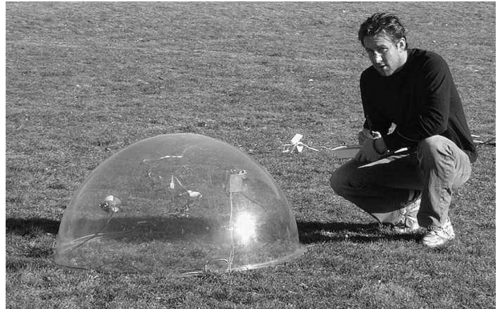
Figure 2. Author Bill Paul and the ET chamber used to measure actual evapotranspiration.
