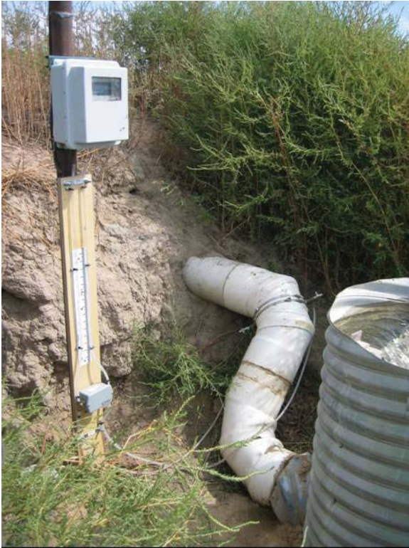
A low-cost flow measurement device using pressure differences on the inside and outside of a pipe elbow bend to determine flow rate.
