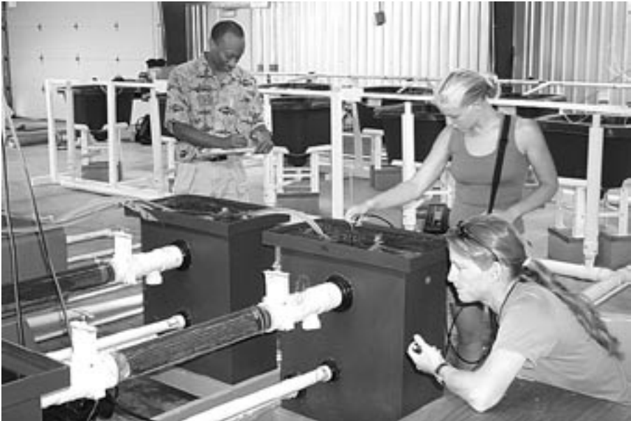
From left: Chris Myrick, Department of Fishery and Wildlife Biology, graduate student Ashley Ficke and summer intern Cloelle Sausville-Giddings are investigating various types of fish ladders and whether they allow fish to move upstream. Results will be used to develop design criteria for fish passage structures.
