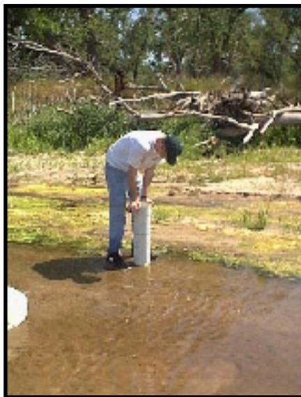
Figure 1. Field measuring the streambed permeability in the South Platte River.
