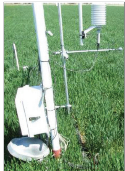
View of the lysimeter looking to the southeast. The net radiometer, infrared thermometer, and temperature/humidity sensor are shown mounted above the lysimeter.
