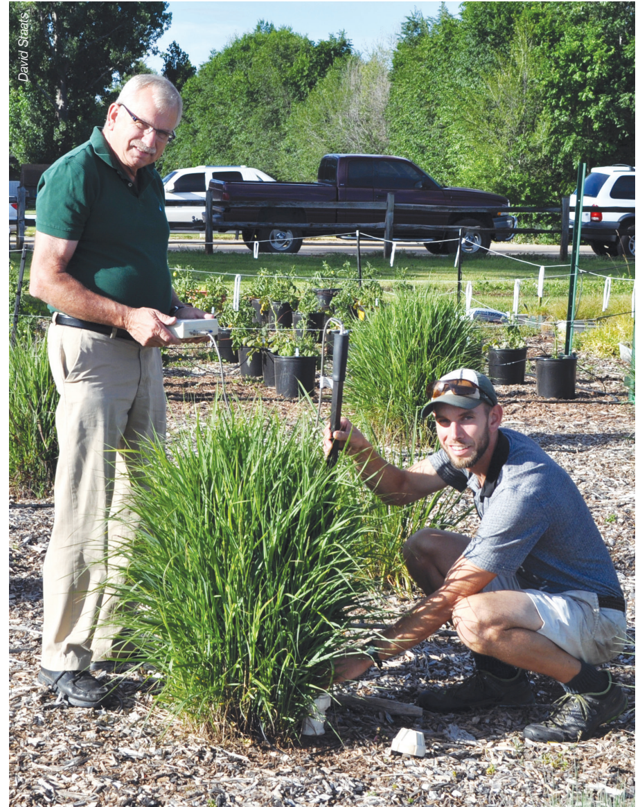
Sam Hagopian and advisor James Klett use frequency domain reflectometry (FDR) to determine where the plant accesses water (vertically), as well as where the plant ceases to access water, as part of a plant stress and aesthetics watering study.
