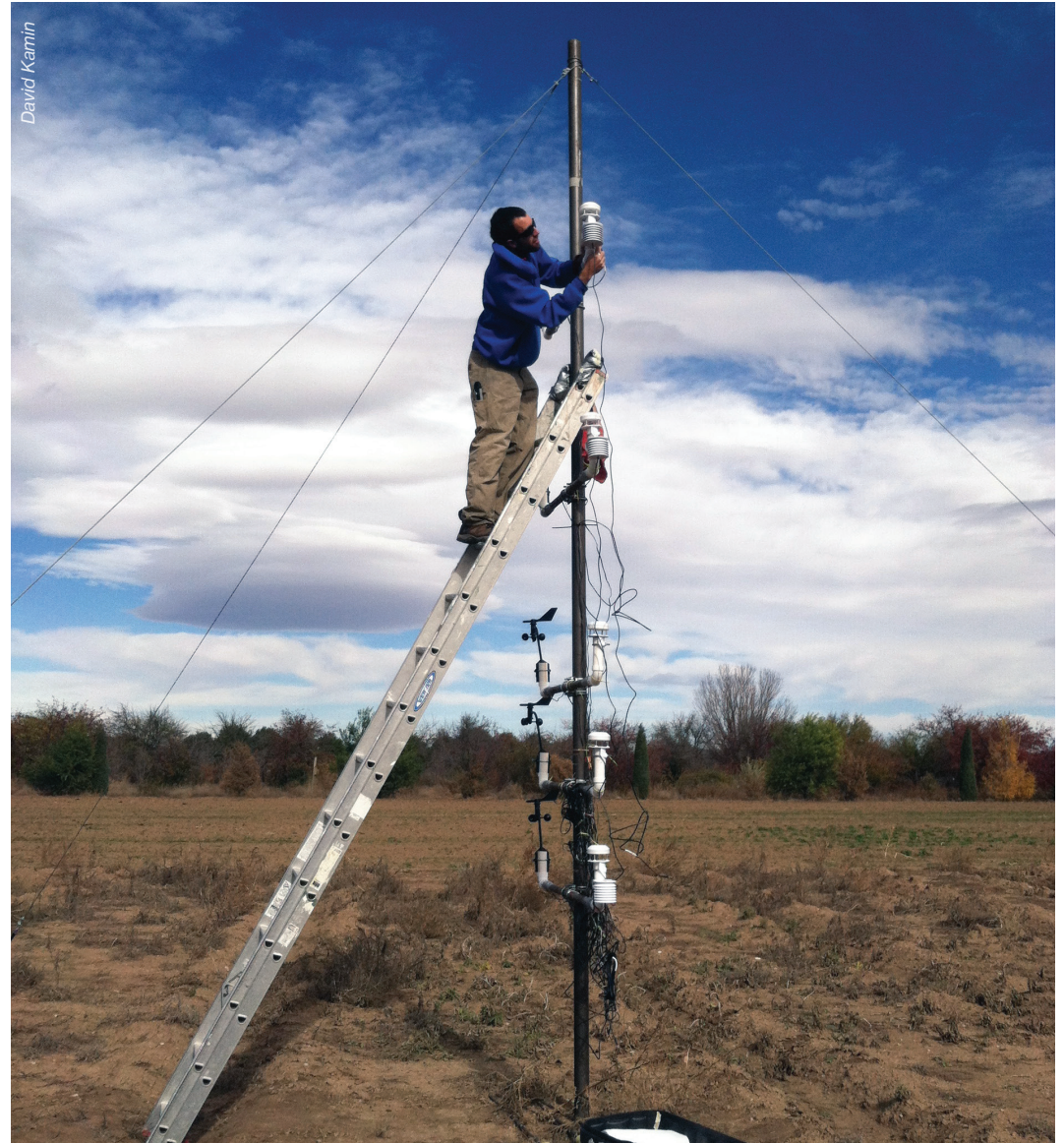
Student researcher David Kamin adjusts instruments on the meteorological tower, which records temperature, humidity, and wind speed.
