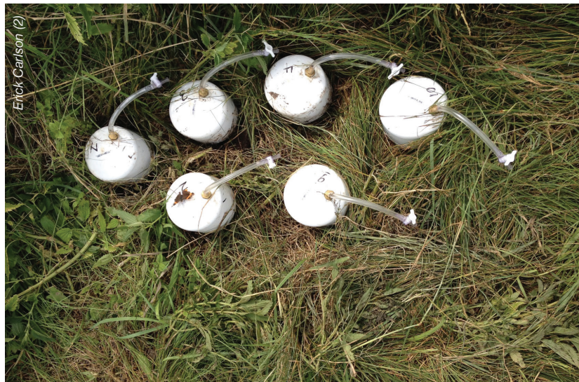
Soil incubation chamber in the field near Gilcrest. Notice the gas exchange port and stockcock for taking samples.
