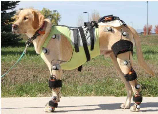
Figure 1. Picture of dog fitted for the study depicting 2 IMUs for thoracic limb and 4 for pelvic limb data acquisition.
