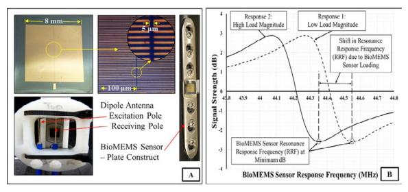
Figure 1. (A) Macro and micro digital images of the bioMEMS sensor, digital image of dipole antenna placed over the bioMEMS sensor; digital image of the BioMEMS sensor – locking plate construct. (B) Characteristic curves of measured signal strength (dB) versus the resonance response frequency (RRF) under applied loading demonstrating the shift in the RRF due to different load magnitudes imparted on the bioMEMS sensor.
