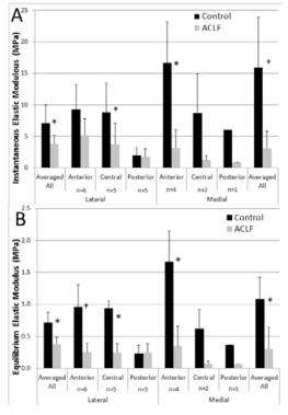
Figure 3. A) Instantaneous elastic modulus of the menisci B) equilibrium elastic modulus of the menisci (mean with standard deviation) \* denotes p<0.05 and + denotes p<0.1 between control and ACLF.
