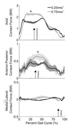
Figure 3. Compressive (top), anterior-posterior (middle), and medial-lateral (bottom) tibiofemoral contact forces predicted from the sheep hind limb musculoskeletal model during treadmill walking at 0.25m•s-1 (black-solid line) and 0.75m•s-1 (graydashed line). The shaded regions represent ±SD. The asterisk depicts a significant difference in peak forces between the slower and faster speeds.
