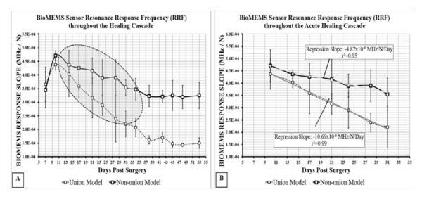
Figure 2. (A) BioMEMS sensor's mean (w/ one standard deviation error bars) temporal RRF response observed under loading during the healing cascade in an ovine metatarsal model. (B) The response during the acute healing phase (7-30 days post-surgery) demonstrated a statistically significant difference (p = 0.01) between the union (-10.69 ± 1.79 [Hz/N]/Day) and non-union (-4.87 ± 0.59 [Hz/N]/Day) models, indicating a substantial temporal reduction in hardware strain in the union model.
