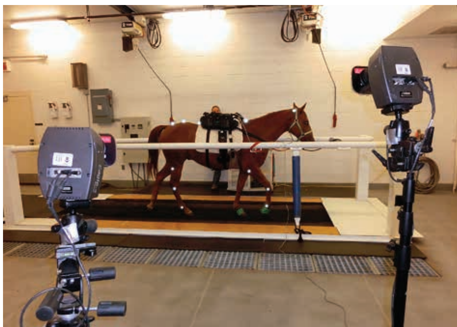
Fig. 2 (below): A horse with the weighted, instrumented saddle on the high-speed treadmill with cameras in the foreground that measure spinal and limb movements via attached reflective markers.
