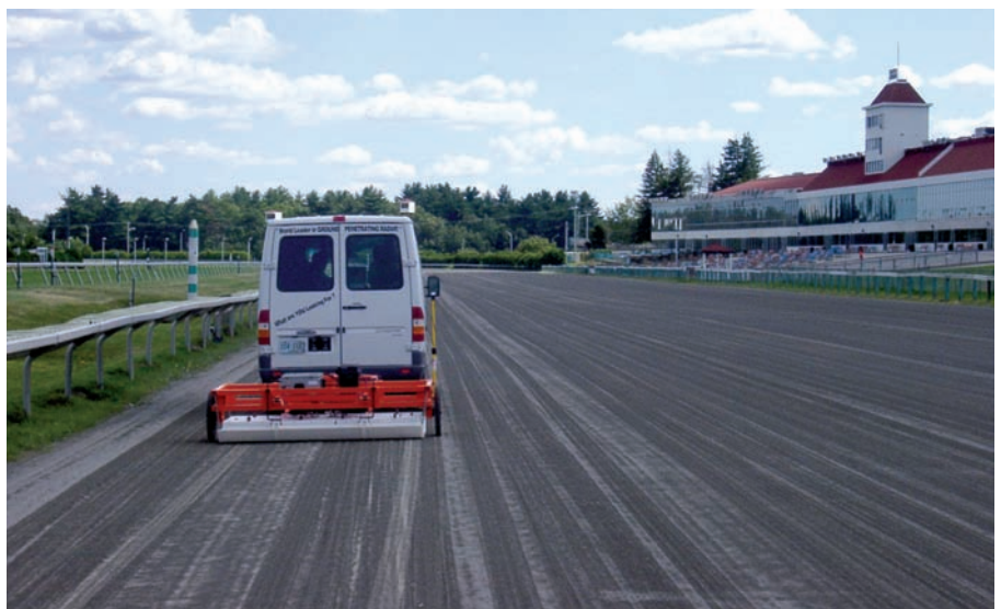
Geophysical Survey Systems ground penetrating radar test of a harness racing track in New Hampshire.
