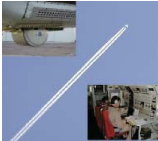
Figure 4. The NASA DC-8 on a high-altitude (39,000' MSL) AIRSAR, POLSCAT, and PSR flight line over North Park. Inset, upper left: AIRSAR antenna (upper structure) and PSR instrument (lower drum-shaped instrument) mounted on the DC-8. Inset, lower right: NASA flight crew at work. (Inset-photos credit: Koni Steffen).
