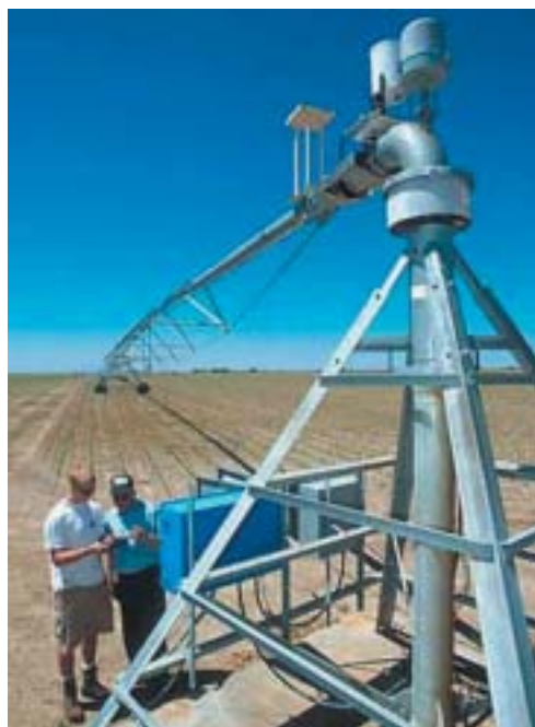
Ryan Younkin and Dale Heerman program irrigations for an automated center pivot sprinkler system near Wiggins, Colo. Photo courtesy Information Staff, USDA-Agricultural Research Service, Beltsville, Md.
