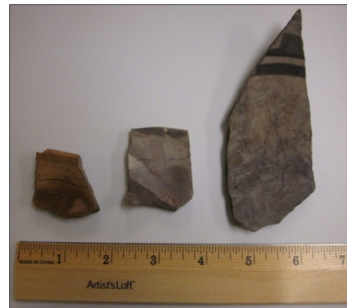
Figure 7: Discoloration as a result of cranberry sauce treatment (left to right): glaze, white, and biscuit ware.
