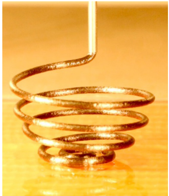
Photo: Net-zero 3D printing of carbon fiber composites in midair Courtesy of Mostafa Yourdkhani
