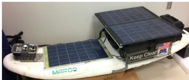
Figure 1. MARCo autonomous unmanned surface vehicle.
