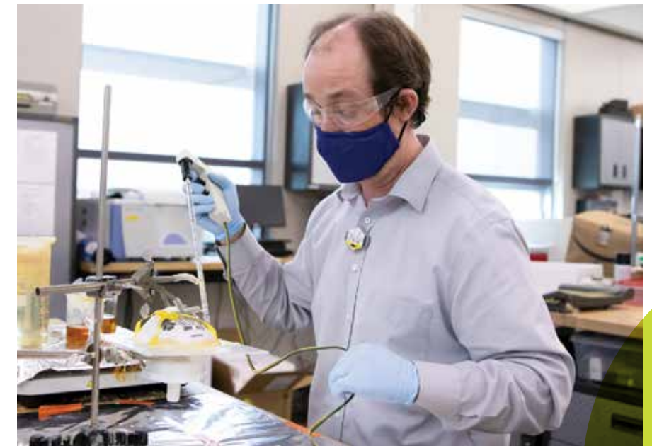
Christian L'Orange seals a mask to a frame with beeswax to prepare it for testing.
