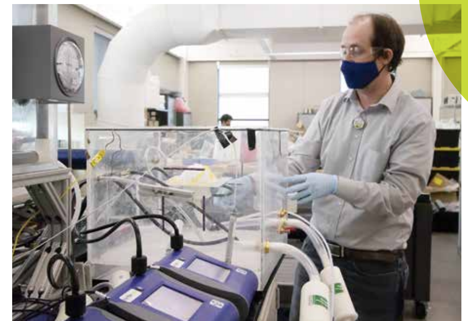
During testing, researchers monitor values of particle filtration efficiency for each mask.
