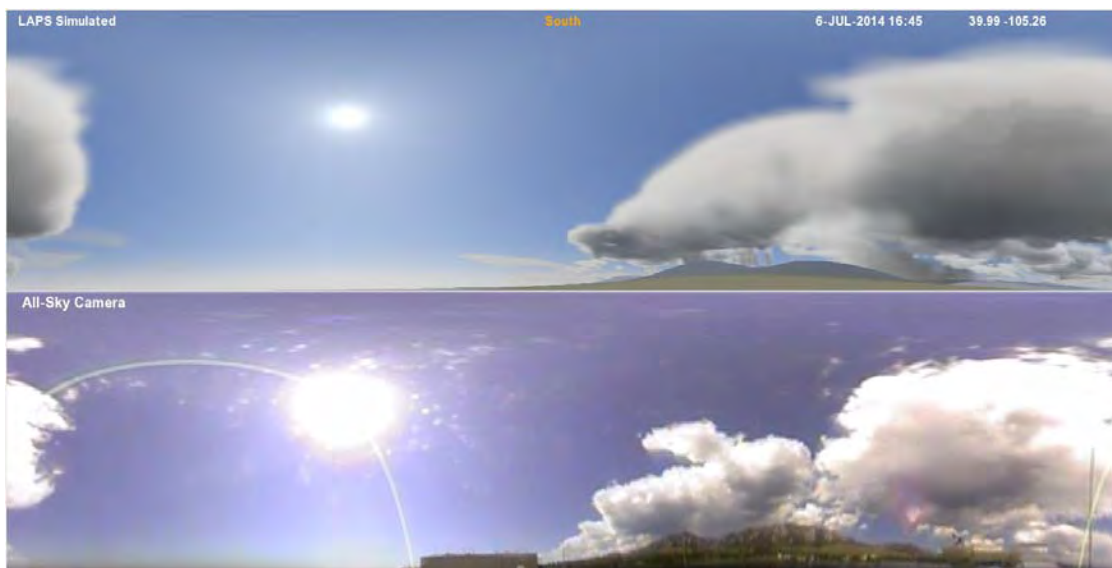
Figure 1. In these 360 degree panoramic views, the top is a simulated LAPS image and bottom is a remapped camera image from an all-sky camera maintained by the Earth Systems Research Laboratory. South is at the center of each image and north is at the edges.
